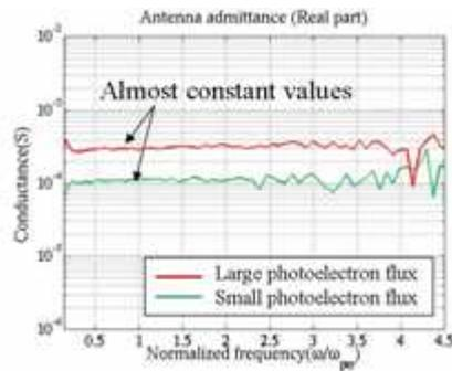
Figure 21: Antenna conductance as function of frequency for the cases of large and small photoelectron fluxes, which is obtained by the Particle-In-Cell simulations.
